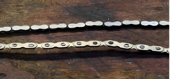
Lastly, I had a triple fussee that broke a chain. Looked in the bottom of the clock and saw a few loose links so I thought I would just order a new chain. (\$83.50US) When the new chain arrived, bottom one in the above picture, I was really disappointed. It was so crudely made that I couldn't bring myself to use it. Ended up splitting a link, making a new pin and then riveting it all back together. So far everything's holding together. Knock on wood.
