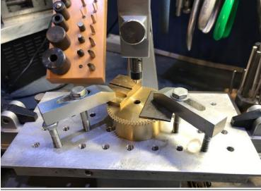
I had to make a barrel for a German Westminster Chime clock that I bought quite some time ago. At one time, someone tried to very crudely replace 3 broken teeth with some filed down bolts inserted in place of the teeth. (Top left picture). The barrel also had a few bent teeth as well, so a new barrel was begun. Top right is the barrel in the lathe, and then the finished barrel getting a proper bushing installed.
